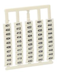
DINnector marking tag, 6 x 12mm, numbered 401-450 (10 of each number). Package of 500. For use with DN-T10-A, DN-D10-A, DN-T8 or DN-F6 series terminal block.
