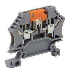
DINnector screw disconnect terminal block, accepts wire size 22-12 AWG, gray, 20A, 35mm DIN rail mount, 10kA SCCR. Package of 10.
