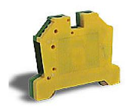
DINnector screw grounding terminal block, accepts wire size 20-6 AWG, green and yellow, 35mm DIN rail mount, 10kA SCCR. Package of 50. Use to mechanically and electrically connect wires to 35mm DIN rail through the clamping foot.
