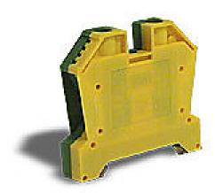
DINnector screw grounding terminal block, accepts wire size 14-4 AWG, green and yellow, 35mm DIN rail mount, 10kA SCCR. Package of 25. Use to mechanically and electrically connect wires to 35mm DIN rail through the clamping foot.
