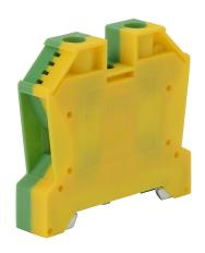
DINnector screw grounding terminal block, accepts wire size 14-4 AWG, green and yellow, 35mm DIN rail mount, 10kA SCCR. Package of 8. Use to mechanically and electrically connect wires to 35mm DIN rail through the clamping foot.
