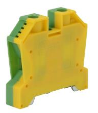
DINnector screw grounding terminal block, accepts wire size 14-4 AWG, green and yellow, 35mm DIN rail mount, 10kA SCCR. Package of 8. Use to mechanically and electrically connect wires to 35mm DIN rail through the clamping foot.
