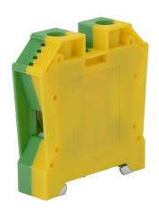
DINnector screw grounding terminal block, accepts wire size 14-1/0 AWG, green and yellow, 35mm DIN rail mount, 10kA SCCR. Package of 5. Use to mechanically and electrically connect wires to 35mm DIN rail through the clamping foot.
