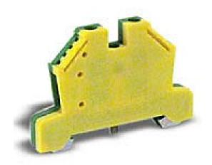
DIN*nector* screw grounding terminal block, accepts wire size 24-10 AWG, green and yellow, 35mm DIN rail mount, 10kA SCCR. Package of 10. Use to mechanically and electrically connect wires to 35mm DIN rail through the clamping foot.
