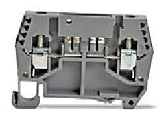
DINnector screw circuit protection terminal block, accepts wire size 24-10 AWG, gray. Package of 50. 25A when used as a disconnect; 10A when used with a DN-SUPP-nn.
