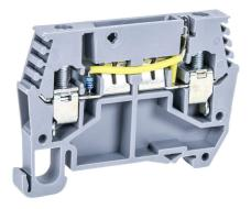
DINnector screw circuit protection terminal block, accepts wire size 24-10 AWG, gray, 24 VAC/VDC LED indicator(s). Package of 50. 25A when used as a disconnect; 10A when used with a DN-SUPP-nn.
