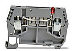
DINnector screw circuit protection terminal block, accepts wire size 24-10 AWG, gray, 24 VAC/VDC LED indicator(s). Package of 5. 25A when used as a disconnect; 10A when used with a DN-SUPP-nn.
