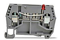
DINnector screw circuit protection terminal block, accepts wire size 24-10 AWG, gray, 12 VAC/VDC LED indicator(s). Package of 5. 25A when used as a disconnect; 10A when used with a DN-SUPP-nn.
