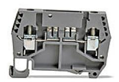
DINnector screw circuit protection terminal block, accepts wire size 24-10 AWG, gray. Package of 5. 25A when used as a disconnect; 10A when used with a DN-SUPP-nn.
