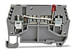
DINnector screw circuit protection terminal block, accepts wire size 24-12 AWG, gray, 24 VAC/VDC LED indicator(s). Package of 5. 20A when used as a disconnect; 10A when used with a DN-SUPP-nn.
