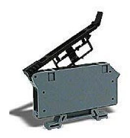
DIN*nector* screw circuit protection terminal block, accepts wire size 20-6 AWG, gray, 30A, 35mm DIN rail mount, 10kA SCCR. Package of 25. For use with ABC, AGC, MDA and MDL series fuses.
