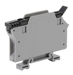
DINnector screw circuit protection terminal block, accepts wire size 20-6 AWG, gray, 30A, 35mm DIN rail mount, 10kA SCCR. Package of 7. For use with ABC, AGC, MDA and MDL series fuses.
