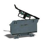
DINnector screw circuit protection terminal block, blown fuse indicator, accepts wire size 20-6 AWG, gray, 30A, 24 VAC/VDC LED indicator(s), 35mm DIN rail mount, 10kA SCCR. Package of 10. For use with ABC, AGC, MDA and MDL series fuses.
