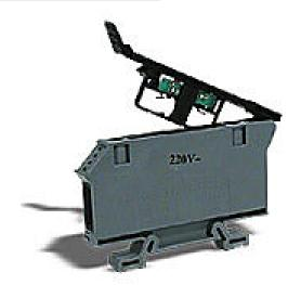
DINnector screw circuit protection terminal block, blown fuse indicator, accepts wire size 20-6 AWG, gray, 30A, 220 VAC/VDC LED indicator(s), 35mm DIN rail mount, 10kA SCCR. Package of 10. For use with ABC, AGC, MDA and MDL series fuses.
