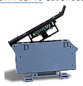
DINnector screw circuit protection terminal block, blown fuse indicator, accepts wire size 20-6 AWG, gray, 30A, 110 VAC/VDC LED indicator(s), 35mm DIN rail mount, 10kA SCCR. Package of 10. For use with ABC, AGC, MDA and MDL series fuses.
