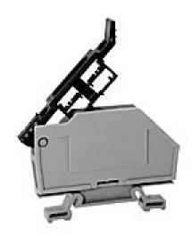
DINnector screw circuit protection terminal block, accepts wire size 24-10 AWG, gray, 15A, 35mm DIN rail mount, 10kA SCCR. Package of 50. For use with GMA, GMC, S500 and S506 series fuses.
