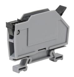
DINnector screw circuit protection terminal block, accepts wire size 24-10 AWG, gray, 6.3A, 35mm DIN rail mount, 10kA SCCR. Package of 10. For use with GMA, GMC, S500 and S506 series fuses.
