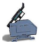
DINnector screw circuit protection terminal block, blown fuse indicator, accepts wire size 24-10 AWG, gray, 6.3A, 24 VAC/VDC LED indicator(s), 35mm DIN rail mount, 10kA SCCR. Package of 10. For use with GMA, GMC, S500 and S506 series fuses.
