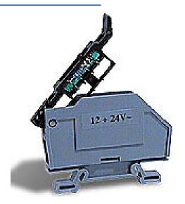
DINnector screw circuit protection terminal block, blown fuse indicator, accepts wire size 24-10 AWG, gray, 15A, 24 VAC/VDC LED indicator(s), 35mm DIN rail mount, 10kA SCCR. Package of 10. For use with GMA, GMC, S500 and S506 series fuses.
