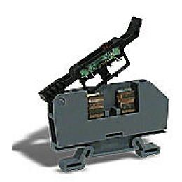
DINnector screw circuit protection terminal block, blown fuse indicator, accepts wire size 24-10 AWG, gray, 15A, 110 VAC/VDC LED indicator(s), 35mm DIN rail mount, 10kA SCCR. Package of 10. For use with GMA, GMC, S500 and S506 series fuses.
