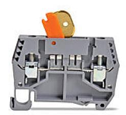
DINnector screw disconnect terminal block, accepts wire size 24-10 AWG, gray, 25A, 35mm DIN rail mount, 10kA SCCR. Package of 50.
