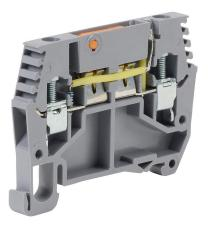
DINnector screw disconnect terminal block, power indicator, accepts wire size 24-10 AWG, gray, 25A, 24 VAC/VDC LED indicator(s), 35mm DIN rail mount, 10kA SCCR. Package of 10.
