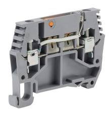
DINnector screw disconnect terminal block, power indicator, accepts wire size 24-10 AWG, gray, 25A, 12 VAC/VDC LED indicator(s), 35mm DIN rail mount, 10kA SCCR. Package of 10.
