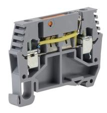
DINnector screw disconnect terminal block, power indicator, accepts wire size 24-12 AWG, gray, 20A, 24 VAC/VDC LED indicator(s), 35mm DIN rail mount, 10kA SCCR. Package of 10.
