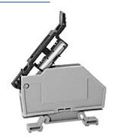
DINnector screw disconnect terminal block, accepts wire size 24-10 AWG, gray, 30A, 35mm DIN rail mount, 10kA SCCR. Package of 50.
