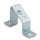
AutomationDirect angled DIN rail support bracket, 49mm, zinc plated steel. Package of 50. For use with 35mm DIN rail. M6 metric threaded hole and 5mm unthreaded mounting hole.
