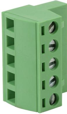
DINnector terminal plug, 5-pole, accepts wire size 22-14 AWG, green, 12A, 300V rated (UL), top wire entry with terminal screw 90 degrees from entry. For use with DN-EMXM1 or DN-EMXDV series terminal block. Package of 100.
