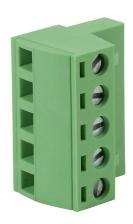
DINnector terminal plug, 5-pole, accepts wire size 22-14 AWG, green, 12A, 300V rated (UL), top wire entry with terminal screw 90 degrees from entry. For use with DN-EMXM1 or DN-EMXDV series terminal block. Package of 100.
