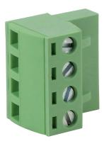
DINnector terminal plug, 4-pole, accepts wire size 22-14 AWG, green, 12A, 300V rated (UL), top wire entry with terminal screw 90 degrees from entry. For use with DN-EMXM1 or DN-EMXDV series terminal block. Package of 10.
