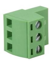
DINnector terminal plug, 3-pole, accepts wire size 22-14 AWG, green, 12A, 300V rated (UL), top wire entry with terminal screw 90 degrees from entry. For use with DN-EMXM1 or DN-EMXDV series terminal block. Package of 200.
