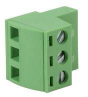
DINnector terminal plug, 3-pole, accepts wire size 22-14 AWG, green, 12A, 300V rated (UL), top wire entry with terminal screw 90 degrees from entry. For use with DN-EMXM1 or DN-EMXDV series terminal block. Package of 10.
