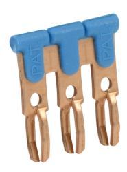
DINnector terminal block jumper, push-in type, 3-pole, blue, 20A, 300V rated (UL). Package of 100. For use with DN-TL14-A, DN-TL14S-A, DN-TL14SLP or DN-14SLN-A series terminal block.
