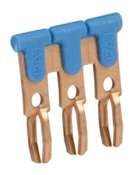
DINnector terminal block jumper, push-in type, 3-pole, blue, 20A, 300V rated (UL). Package of 25. For use with DN-TL14-A, DN-TL14S-A, DN-TL14SLP or DN-14SLN-A series terminal block.
