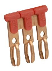
DINnector terminal block jumper, push-in type, 3-pole, red, 20A, 300V rated (UL). Package of 100. For use with DN-TL14-A, DN-TL14S-A, DN-TL14SLP or DN-14SLN-A series terminal block.
