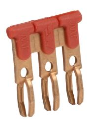
DINnector terminal block jumper, push-in type, 3-pole, red, 20A, 300V rated (UL). Package of 25. For use with DN-TL14-A, DN-TL14S-A, DN-TL14SLP or DN-14SLN-A series terminal block.
