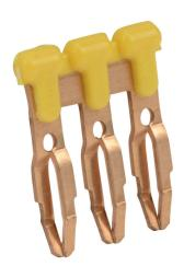
DINnector terminal block jumper, push-in type, 3-pole, yellow, 25A, 600V rated (UL). Package of 25. For use with DN-T10-A, DN-D10-A, DN-M10-A or DN-Q10-A series terminal block.
