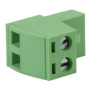
DINnector terminal plug, 2-pole, accepts wire size 22-14 AWG, green, 12A, 300V rated (UL), top wire entry with terminal screw 90 degrees from entry. For use with DN-EMXM1 or DN-EMXDV series terminal block. Package of 10.
