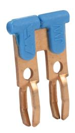
DINnector terminal block jumper, push-in type, 2-pole, blue, 20A, 300V rated (UL). Package of 100. For use with DN-TL14-A, DN-TL14S-A, DN-TL14SLP or DN-14SLN-A series terminal block.
