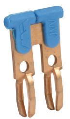
DINnector terminal block jumper, push-in type, 2-pole, blue, 20A, 300V rated (UL). Package of 25. For use with DN-TL14-A, DN-TL14S-A, DN-TL14SLP or DN-14SLN-A series terminal block.
