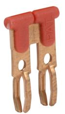
DINnector terminal block jumper, push-in type, 2-pole, red, 20A, 300V rated (UL). Package of 100. For use with DN-TL14-A, DN-TL14S-A, DN-TL14SLP or DN-14SLN-A series terminal block.
