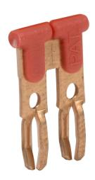
DINnector terminal block jumper, push-in type, 2-pole, red, 20A, 300V rated (UL). Package of 100. For use with DN-TL14-A, DN-TL14S-A, DN-TL14SLP or DN-14SLN-A series terminal block.
