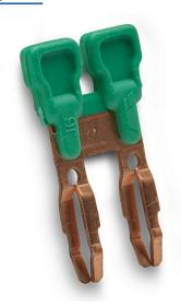
DINnector terminal block jumper, push-in type, 2-pole, green, 30A, 600V rated (UL). Package of 100. For use with DN-Q8-A or DN-Q8B-A series terminal block.
