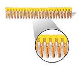
DIN*nector* terminal block jumper, push-in type, 24-pole, yellow, 25A, 600V rated (UL). Package of 5. For use with DN-T10-A, DN-D10-A, DN-M10-A and DN-Q10-A series terminal block.
