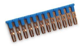
DINnector terminal block jumper, push-in type, 12-pole, blue, 20A, 300V rated (UL). Package of 10. For use with DN-TL14-A, DN-TL14S-A, DN-TL14SLP or DN-14SLN-A series terminal block.
