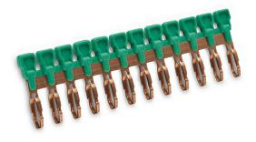
DINnector terminal block jumper, push-in type, 12-pole, green, 30A, 600V rated (UL). Package of 10. For use with DN-Q8-A or DN-Q8B-A series terminal block.
