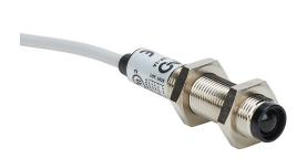
AutomationDirect photoelectric sensor, tubular, threaded, metal housing, through-beam receiver, 4m sensing distance, 10-30 VDC operating voltage, selectable light-on/dark-on, PNP, 4-wire, pigtail.
