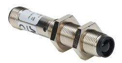
AutomationDirect photoelectric sensor, tubular, threaded, metal housing, through-beam receiver, 4m sensing distance, 10-30 VDC operating voltage, selectable light-on/dark-on, NPN, 4-wire, 4-pin M12 quick-disconnect.
