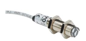
AutomationDirect photoelectric sensor, tubular, threaded, polarized retroreflective, visible red, 2m sensing distance, selectable light-on/dark-on, PNP, teach-in button, 4-wire, pigtail.
