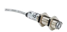
AutomationDirect photoelectric sensor, tubular, threaded, polarized retroreflective, visible red light emission, 2m sensing distance, selectable light-on/dark-on, PNP, teach-in button, 4-wire, pigtail.
