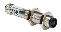
AutomationDirect photoelectric sensor, tubular, threaded, metal housing, through-beam emitter, infrared, 4m sensing distance, 10-30 VDC operating voltage, NPN, 3-wire, 4-pin M12 quick-disconnect.
