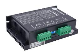
Leadshine AC/DC microstepping stepper drive, 7.2A per phase, 2-phase output, 24-70 VAC/24-90 VDC, bipolar, position mode, 400 to 51200 steps per revolution.
